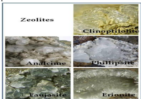
Fig.1. Minerals with zeolite structure (Source: Mastinu et al. , 2019)
